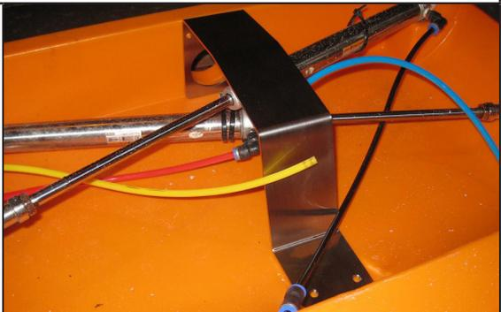
Replace ram protector bracket and insert the necessary screws.
