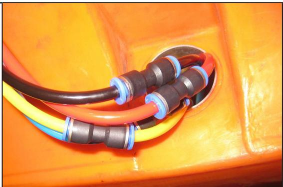
Disconnect air hoses (in roof of drafter unit) by pressing the blue ring on the end of each push-fitting then pull air tube from fitting. Note their original location for future reinstatement.
