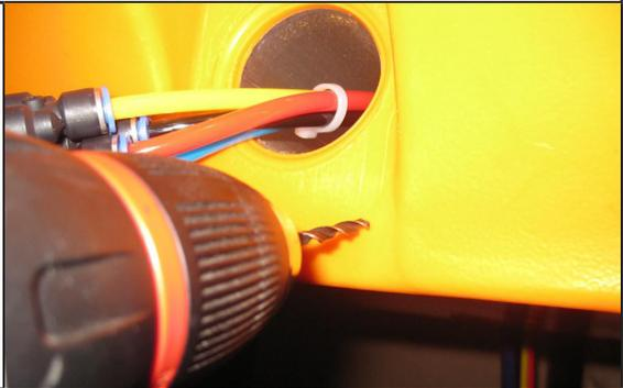
Remove bracket to drill holes with a recommended depth of 15mm.
