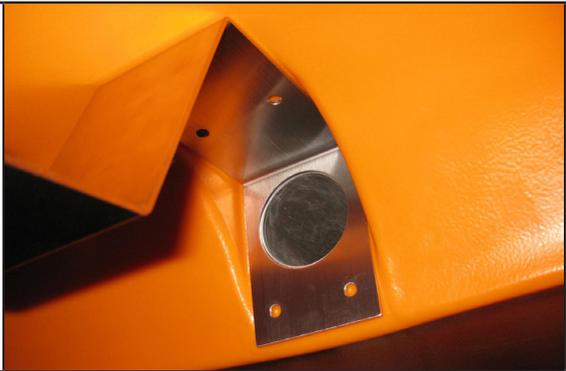
Temporarily place the ram protector bracket inside the roof of the drafter unit and mark the required hole positions on the plastic roof.
